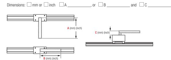
3. Rail Mount Orientation? The force needed to move the load is dependent on the orientation of the load relative to the force of gravity. For example, total required force in the horizontal plane (D) is a function of friction and the force needed for load acceleration ( $F_f + F_a$ ). Total force in the vertical plane is a function of friction, load acceleration, and gravity ( $F_f + F_a + F_g$ ).
