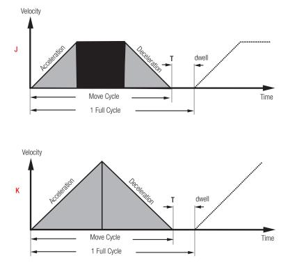
If using a *trapezoidal* (J) or *triangular* (K) move profile, the following is needed.
